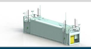
To meet UL2085 the requirement is for 3 inches or 75mm of insulation on all faces of the tank, including the roof and floor. This is sandwiched between the inner and outer skins.
